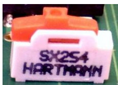
Switch position left (delivery status)
